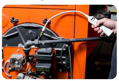
The ecom-LSG leak detector is designed for the quick and reliable locating of leaks in gas installations. Reverse to leak detection sprays, which can swell seals made from, for example, hemp and thus seal them again after a short time, leak detection with the ecom-LSG is simple and unproblematic.
