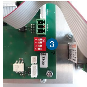
1 Knurled screw 2 Front plate 3 DIP switch
